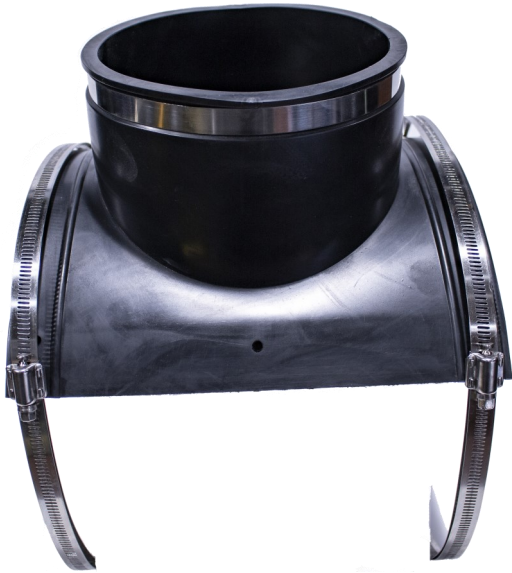
Reducing size Flexible Saddle Tee's include flexible pvc bushing(s) to accommodate size reduction from 4" or 6" down to 1-1/2" for each saddle tee
